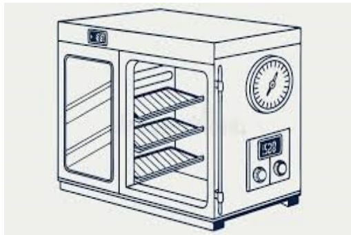
Drying in hot air Oven at 80°C for 7h
